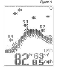
**Speed/Temperature.** The initial screen layout takes one of two basic forms depending on presence of accessories such as Temperature or Speed/Temperature sensors. Figure A shows the default view when the Speed/Temp or Temperature accessory is installed. Figure B shows the default view when no accessory is installed.
